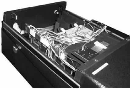
Target drum and illumination lamps are readily accessible by removing the top cover of the case. The drum contains eight permanently-mounted stereoscopic tests.
