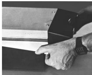
**IMPORTANT NOTICE:** The instrument is held closed by a magnetic latch. To free the latch, place thumbs on top edge of base and press up on bottom of chassis (see illustration).
